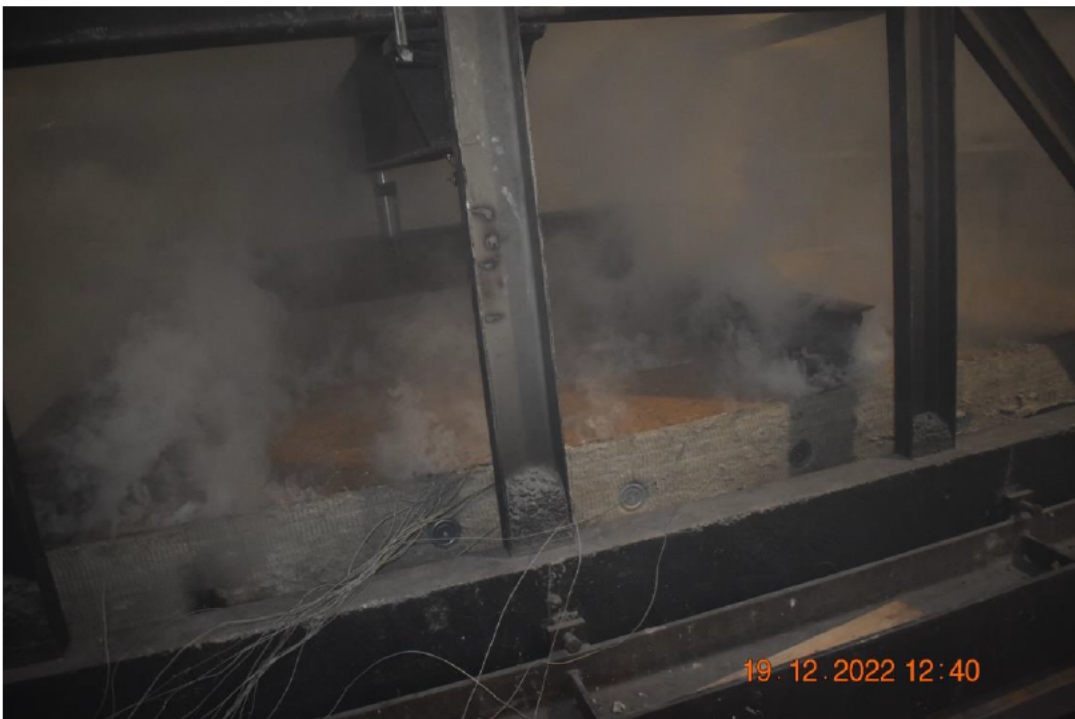
Photo No. 14 Test specimen seen from unexposed side after 43 minutes of testing
