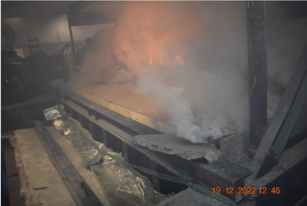
Photo No. 15 Test specimen seen from unexposed side after 49 minutes of testing
