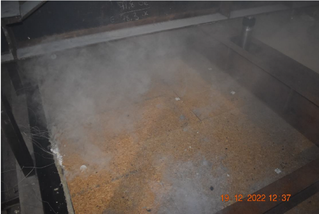
Photo No. 13 Test specimen seen from unexposed side after 40 minutes of testing
