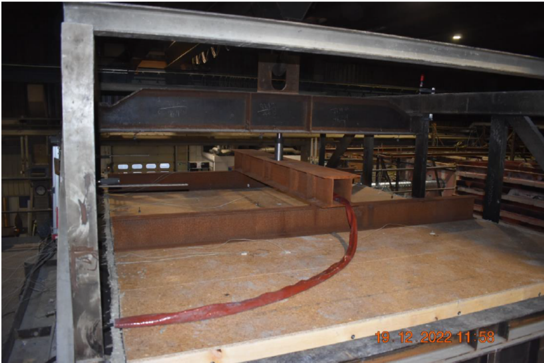
Photo No. 10 Test specimen seen from unexposed side at test start
