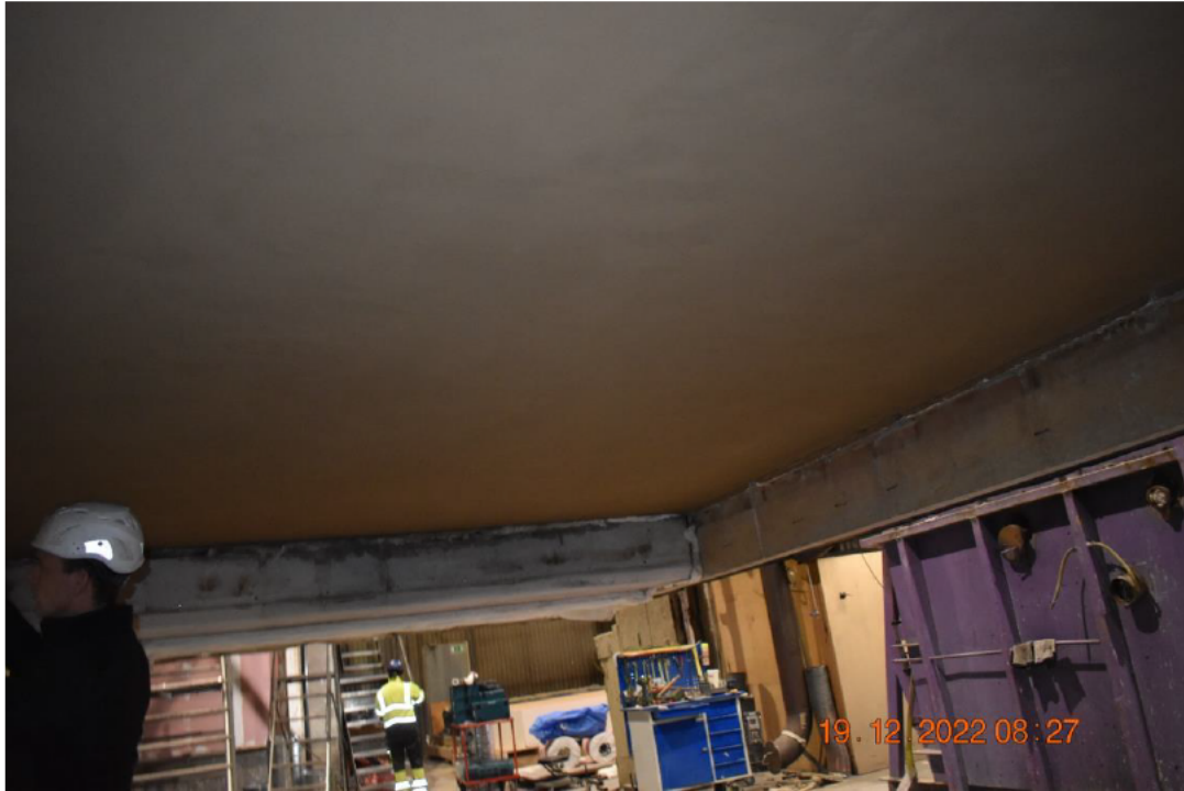
Photo No. 7 Clay plaster and exposed side before test start
