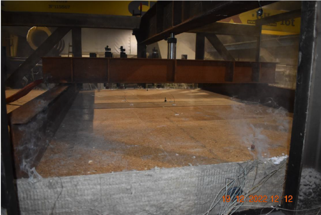
Photo No. 11 Test specimen seen from unexposed side after 15 minutes of testing
