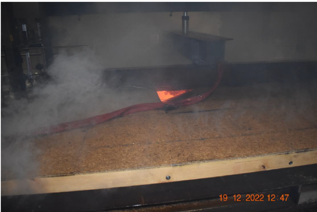
Photo No. 16 Test specimen seen from unexposed side after 50 minutes of testing
