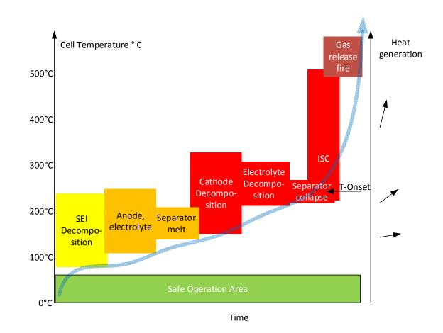
Figure 3: Thermal runaway events at different temperatures.
