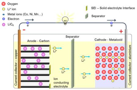
Figure 1: Lithium-ion battery cell during discharge
