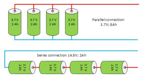
Figure 4: Series and parallel connections of cells.
