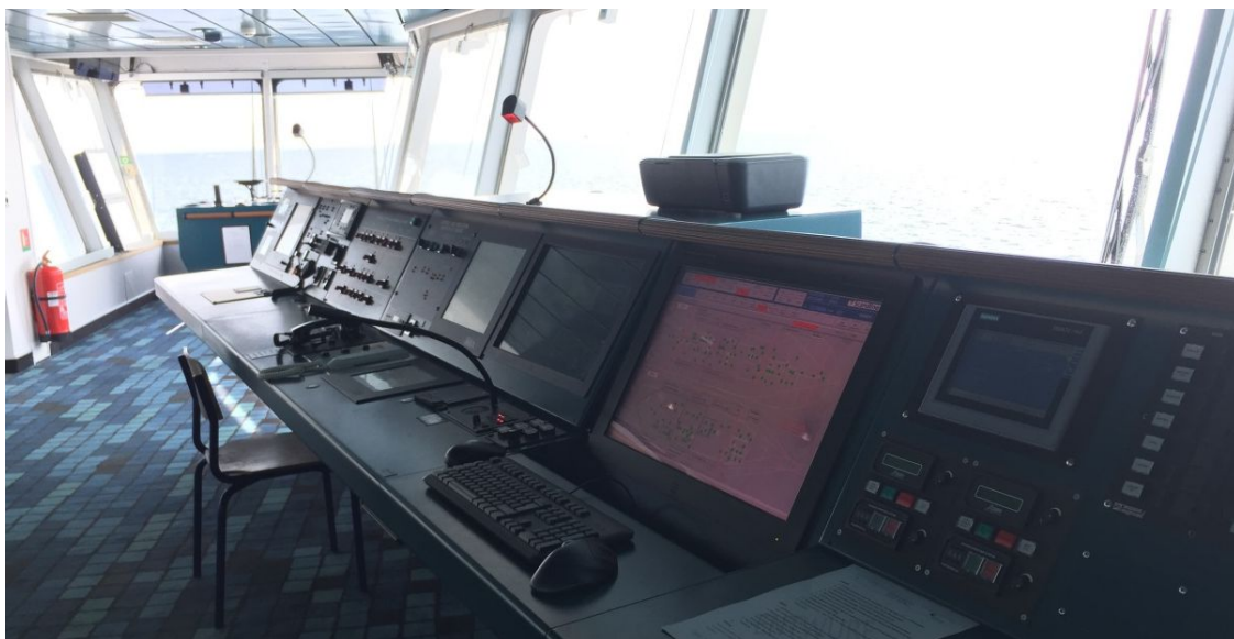
Photo 8. The fire safety control board. There are three systems to back up each other in case of a black out or breach in the technology and communication. To the right are the internet based, digital surveillance system and to the very left is the most basic local wire system.
